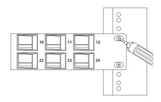
Figure 1. Mounting the panel on a rack.
